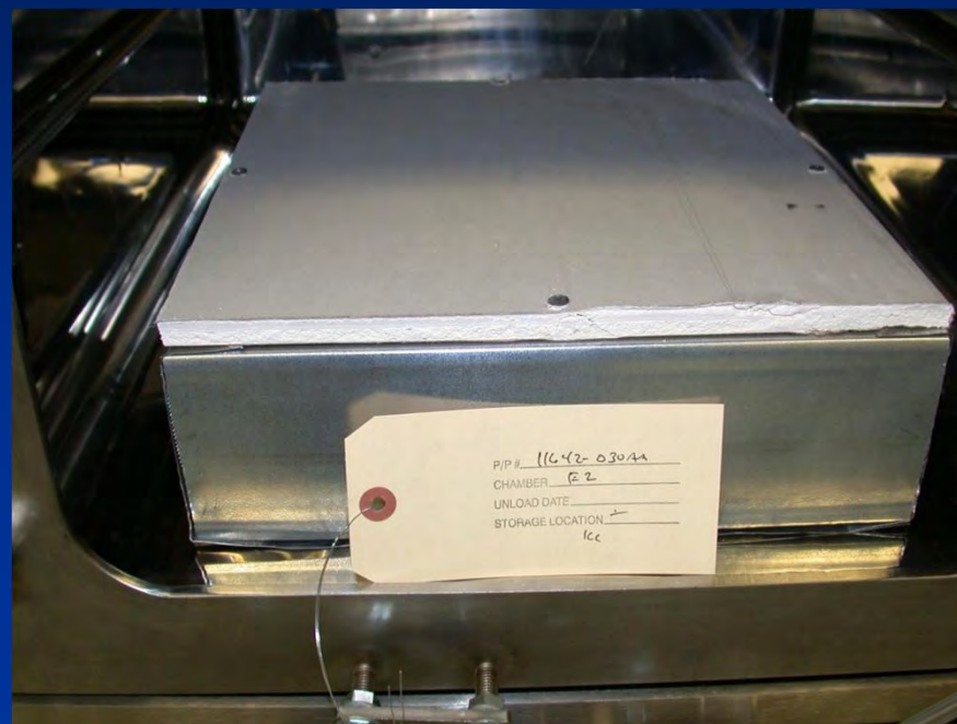
Unfaced fiberglass insulation behind unprepared dry wall
